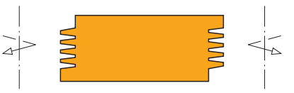
Profile 2 with staggered shoulder cutters
