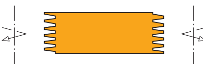
Profile 1 with continuous finger jointing
