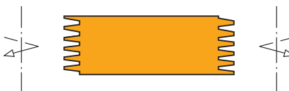
Profile 1 with continuous finger jointing
